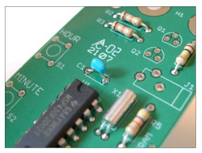
Bend the capacitor wires away from each other to hold it in place.
