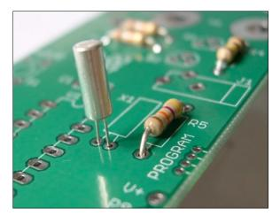
Bend the crystal down to lay in the white square on the board.
