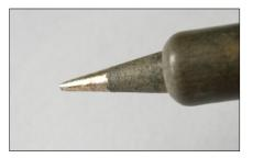
You should have a wet sponge on hand to keep the tip shiny and remove blobs of solder as you work. In extreme cases, you may need to sand the tip clean of solder and oxidization (when it's cool, of course).
