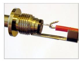
Solder the red wire to the short tab on the chrome plug. Use enough heat and solder
