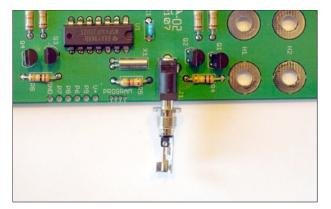
There are two solder connections to make on the plug. Note that there are two tabs on the plug -- a small tab and a long tab. Each tab has a small hole. In the next few steps, we'll attach the battery holder's black wire through the hole in the long tab and the red wire through the hole in the small tab.
