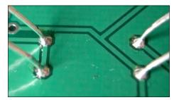
Clip the excess wire from the resistor.
