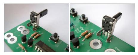
Solder the three small holes on each variable resistor. Soldering the two big holes of each part is optional (and difficult because of the large size of the holes).
