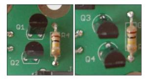
Solder the transistor wires. Be careful not to overheat and damage the transistor. Don't solder for more than five seconds without letting the transistor cool off.
