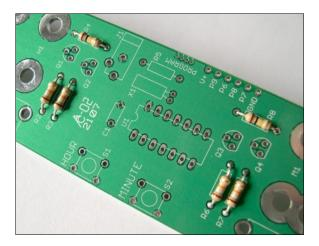
Bend the wires a bit to keep the resistors from falling out.
