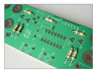
Bend the wires a bit to keep the resistor from falling out.
