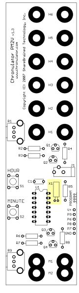
Turn the board over and solder the crystal to the board. To avoid damaging the crystal, don't solder for more than five seconds without letting the crystal cool.
