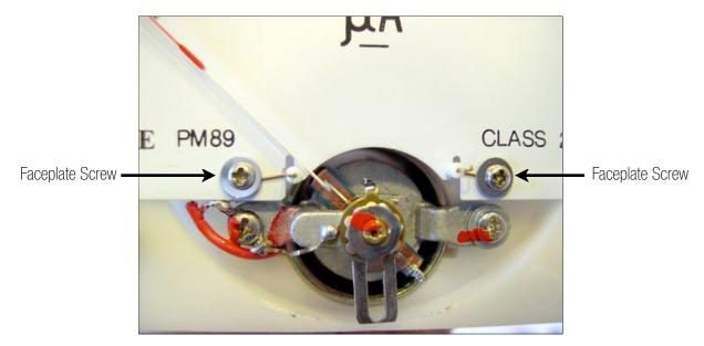
Loosen each of the two faceplate screws about two turns. Rotate the wire bumpers down so they won't be in the way of the artwork when you slide it in.
