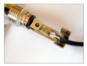
Turn the circuit board over to look at the back side of the plug. There's an indentation in the back side, next to the hole. The metal part of the black wire should lay in that indentation.
