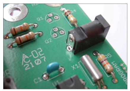
Solder the three pins of the jack. They'll take a fair amount of solder because the holes are big. But don't overdo it. Once you have the hole filled, you're done. It's possible to use so much solder that you create a solder bridge underneath the component, between the pins. (In other words, a short circuit you can't see. Not fun.)
