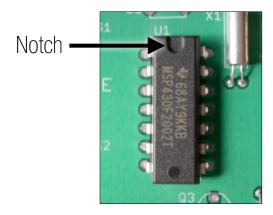
Gently insert the chip into the board. If the chip doesn't drop into the board, you may need to bend the pins of the chip inward slightly so the pins are all parallel to each other.
