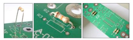
Turn the board over so the resistor wires are accessible. Bend the wires out slightly to keep the resistors from falling out of the board while you're soldering.
