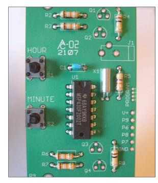
Solder the four pins of each switch.
