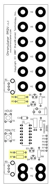
Press the board gently against the table to hold the parts in place. Solder both wires of each resistor to the corresponding metal holes in the board.
