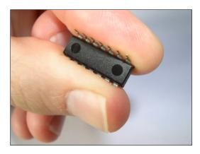
Notice the U-shaped notch at one end of the chip. Also notice the notch in the symbol for U1 on the circuit board. When inserting the chip, be sure the chip is turned so both notches are on the same end.
