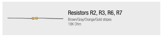
Using your fingers, bend the resistor wires at right angles so both wires are parallel:
