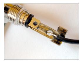
Turn the circuit board over to look at the back side of the plug. There's an indentation in the back side, next to the hole. The metal part of the black wire should lay in that indentation.
