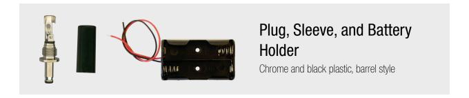
Thread the red and black wires of the battery holder through the black plastic plug sleeve. One end of the sleeve has threads inside. The other end has a smaller hole. The wires go in through the smaller hole and come out on the side with the threaded hole.
