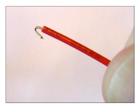
Turn the circuit board over so you can access the short tab. Hook the red wire through the short tab on the chrome plug. Hook the wire from the bottom side so the end of the wire sticks out.
