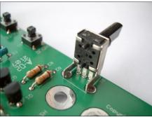
Solder the three small holes on each variable resistor. Soldering the two big holes of each part is optional (and difficult because of the large size of the holes).
